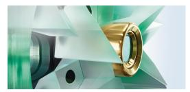
A look at the laser resonator: The mirrors in the optical cavity guide the pump beam emitted by the diodes through the disk crystal multiple times in order to concentrate the laser beam. Picture: TRUMPF
