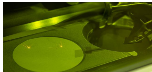
<p><span lang="EN-US">The pulsed laser in TRUMPF's TruPrint 1000 is an excellent choice for creating high-quality surfaces. Its multi-laser capabilities enable highly productive manufacturing processes. (Picture:</span> Steffen Müller-Klenk)</p>
