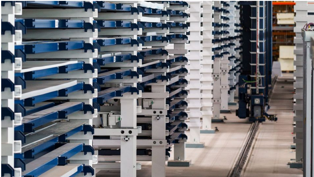
The storage system has 582 storage bays for large-format metal sheets. © Thomas Abe
