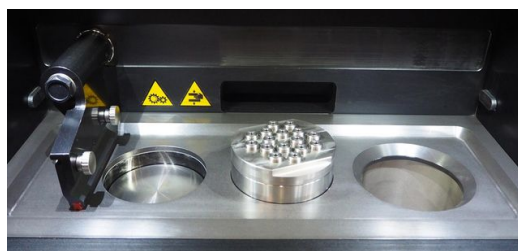
Preforms in TruPrint 1000: A fixture holding preforms in the 3D printer's build chamber
