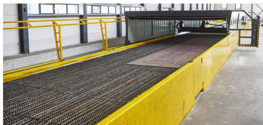
66 Meters – a table this long is perfect for even the largest sheets, and it also creates space for loading and unloading while the machine is cutting (Photos: Norbert Voskens).
