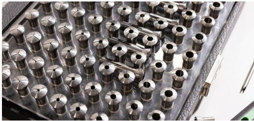
Thanks to robust and flexible tooling setting up the machine with new part holding and aligning the optics takes less than five minutes: Here are the clamping devices for machine retooling.
