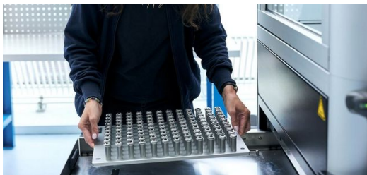
The automation cell is equipped with four drawers. There is space for 960 components. They are loaded and unloaded while the machine is welding.
