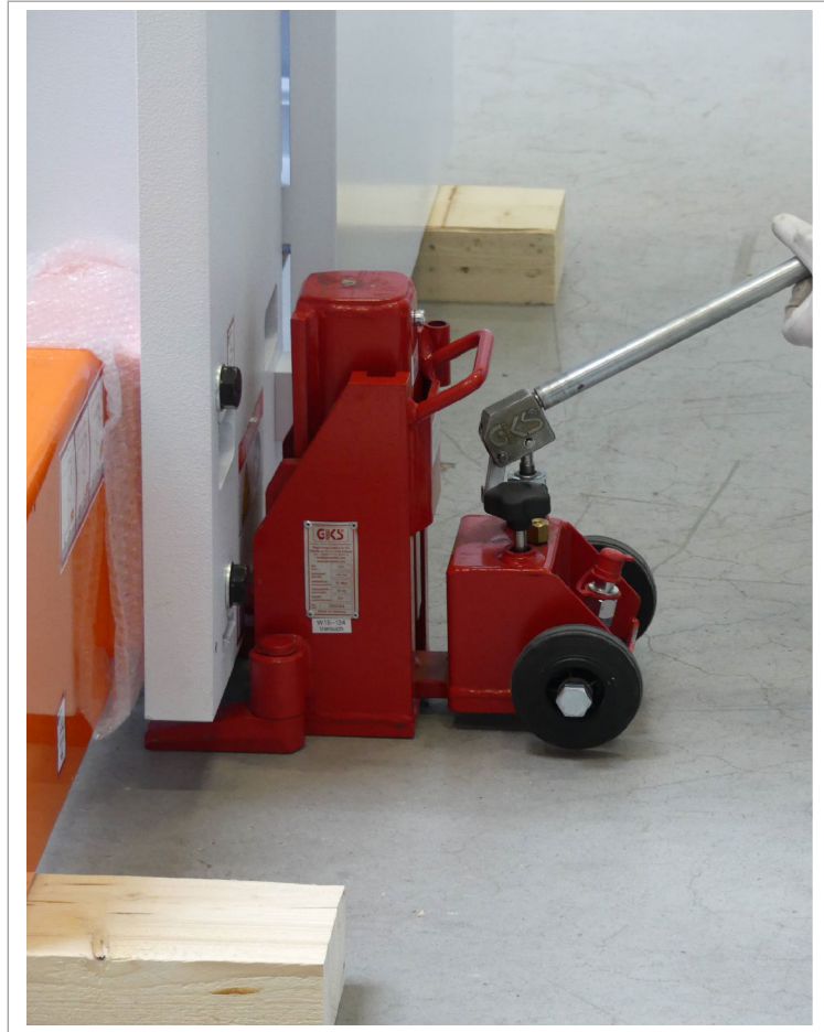
Lowering the machine to 80 mm
