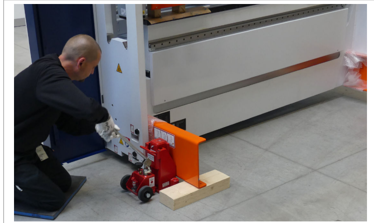
Lowering the left side of the machine to 80 mm
