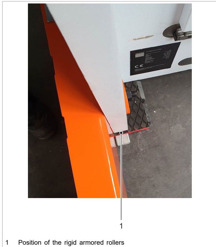
Position of rigid armored roller in relation to machine frame
