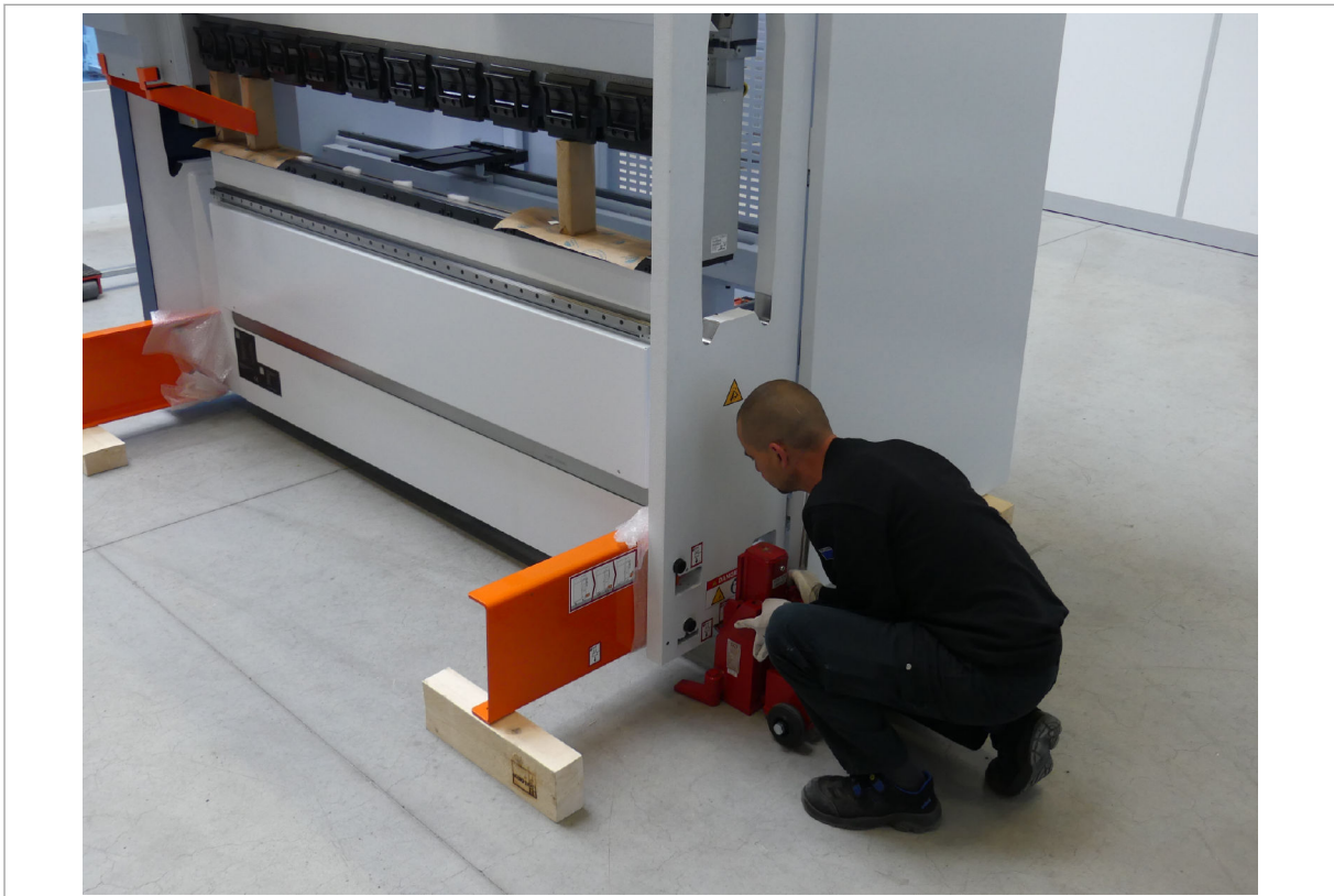
Lowering the right side of the machine to 140 mm
