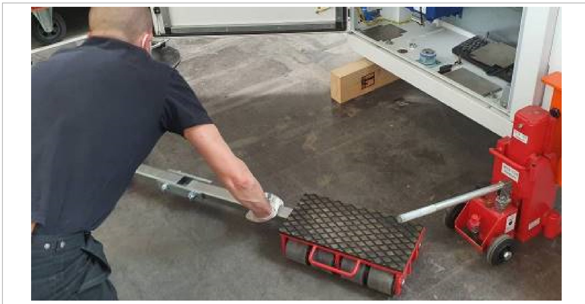
Removing rigid armored rollers
