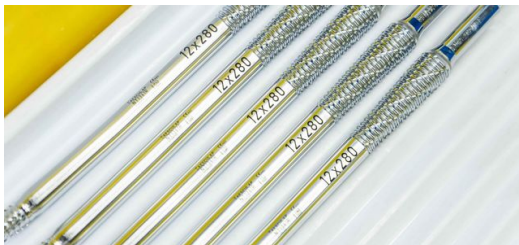
The company uses TruMicro Mark ultrashort pulse lasers from TRUMPF to produce robust and durable markings.
