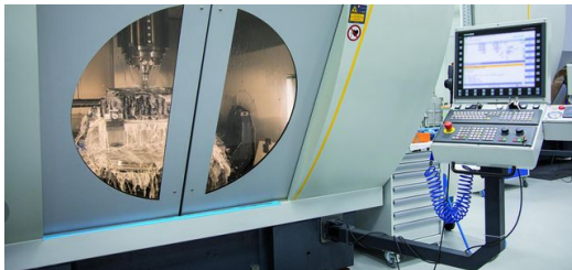
<p><span lang="EN-US">A Zeiss system grinds and polishes a mirror for EUV production.</span></p> – Zeiss
