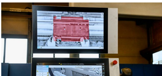
The Part Indicator in action: The system immediately shows whether the bending part is positioned correctly or incorrectly. Red means there is still an error here.
