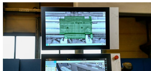
If the Part Indicator shows green, the bending part has been correctly positioned. Thanks to this function, Fischer Maschinenbau has been able to minimize scrap in their sheet metal processing and increase speed.
