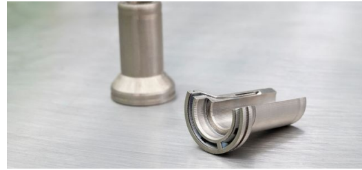
<p>Amorphous metals are produced by flash-freezing molten metals. The atoms solidify in a random arrangement and do not form crystal structures.</p>
