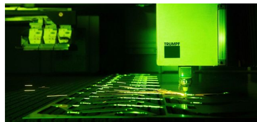
<p>Hans Sanders considers process reliability to be of paramount importance, and he is particularly impressed by the safety features incorporated into the TruLaser Center 7030. As an example, the SmartGate integrated into the brush tables prevents parts from tipping over during the cutting process.</p>
