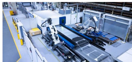
A general view of the TruLaser 8000 Coil Edition: This picture shows how much less sheet metal waste is left over when Fendt cuts from the coil instead of the sheet.
