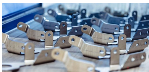
In their own sheet metal processing MERZ processes between 10 and 15 tons of thin sheet daily in a 3-shift operation. A large variety of parts with quantities of 1 to 1,000 as well as a high time pressure are challenges that come with daily work.
