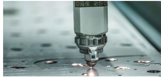
When cutting stainless steel in the thickness range of three to 20 millimeters, DELO needs up to 70 percent less nitrogen with the HighSpeed Eco option.
