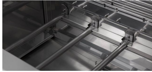
The four stainless steel burner rods in the gas grills are cut on a TRUMPF laser tube cutting machine and each has 144 holes. The hole diameter, which becomes smaller towards the back, guarantees even heating of the entire grill grate.
