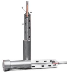
Two additive methods are used to produce the metal pin in the mold: the 3D-printed steel body features cooling channels (1) and contains a fast-cooling copper pin (2) which is built up in layers using LMD and joined to the steel body (3). (Picture: Philipp Reinhard)
