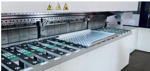
The concept for machining perforated sheets is well thought out. Suction cups, or optional magnetic clamps, can be positioned as desired and secure the sheets firmly. (Picture: KD Busch)
