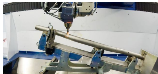
The 3D laser system TruLaser Cell 8030 from TRUMPF can be used to cut out accurate contours, that cannot be inserted before bending because they would otherwise be deformed.
